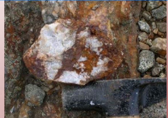
Shaft dump grab samples: to 6.7% copper, 2.92 g/t Au, 443 g/t Ag
