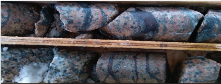
Rateria Zone 2 - Bornite copper veins in drill core.
