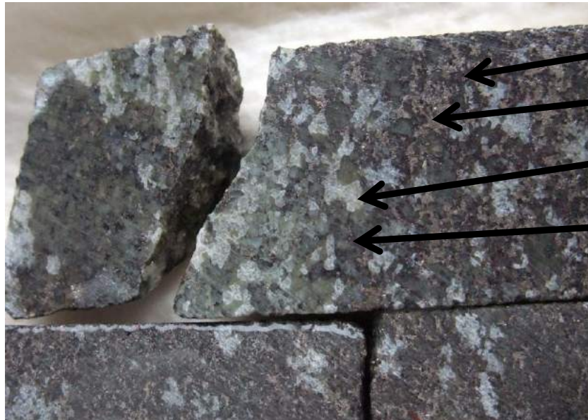
Gangue of calc-silicate minerals: garnet, pyroxene, amphibole, quartz, calcite
