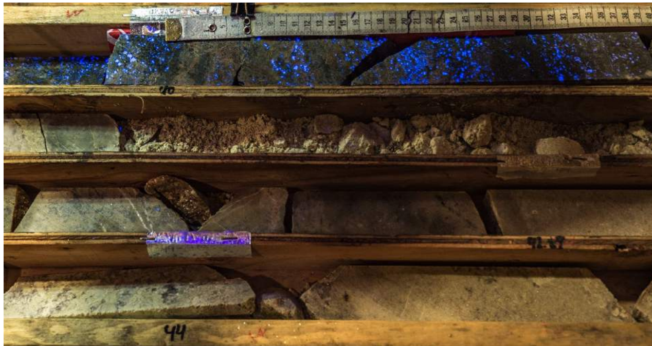
FIGURE 12-1: SCHEELITE MINERALIZATION IN HOLE F13-19 @ 40.10M
