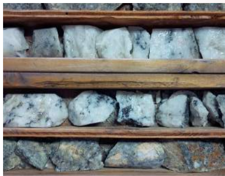
Valley pit drill core (late stage quartz-bornite veins cut phyllic-copper mineralization see Happy Creek's Yubet South)
