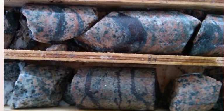
R11-36 K-spar-qtz-sericite veins and bornite. Photo 2.5m 1.11% Cu, 0.46 g/t Au, 0.031% Mo, 0.80 g/t Re
