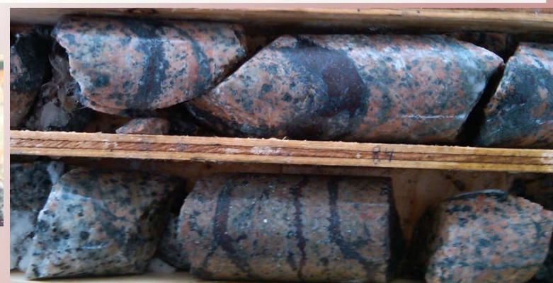
R11-36 K-spar-qtz-sericite bornite veins. Portion of 2.5m with 1.11% Cu, 0.46 g/t Au, 0.031% Mo, 0.80 g/t Re
