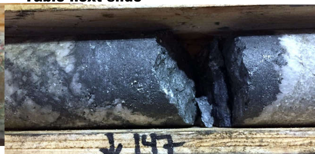
R17-02 Mainly chalcocite: Portion of 5.0m 4.41% Cu, 20.0 g/t Ag, 0.21 g/t Au, 0.031% Mo, 6.86 g/t Re
