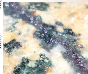
Bornite in quartz green mica, sericite- muscovite veinlet and selective replacement of chlorite altered mafs.
