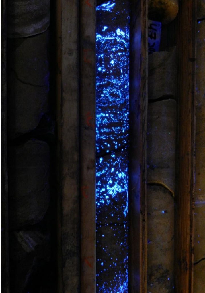
Scheelite, a Tungsten mineral, glows under Shortwave Ultraviolet light in drill core from the Fox Project
