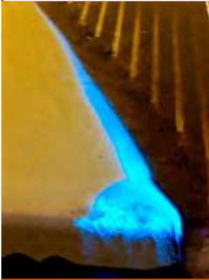
Scheelite (tungsten mineral) under UV light— is recovered by gravity tables in tests at SGS labs.
